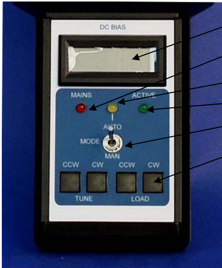
Lower Display/Operator Panel showing Capacitor Position Displays
