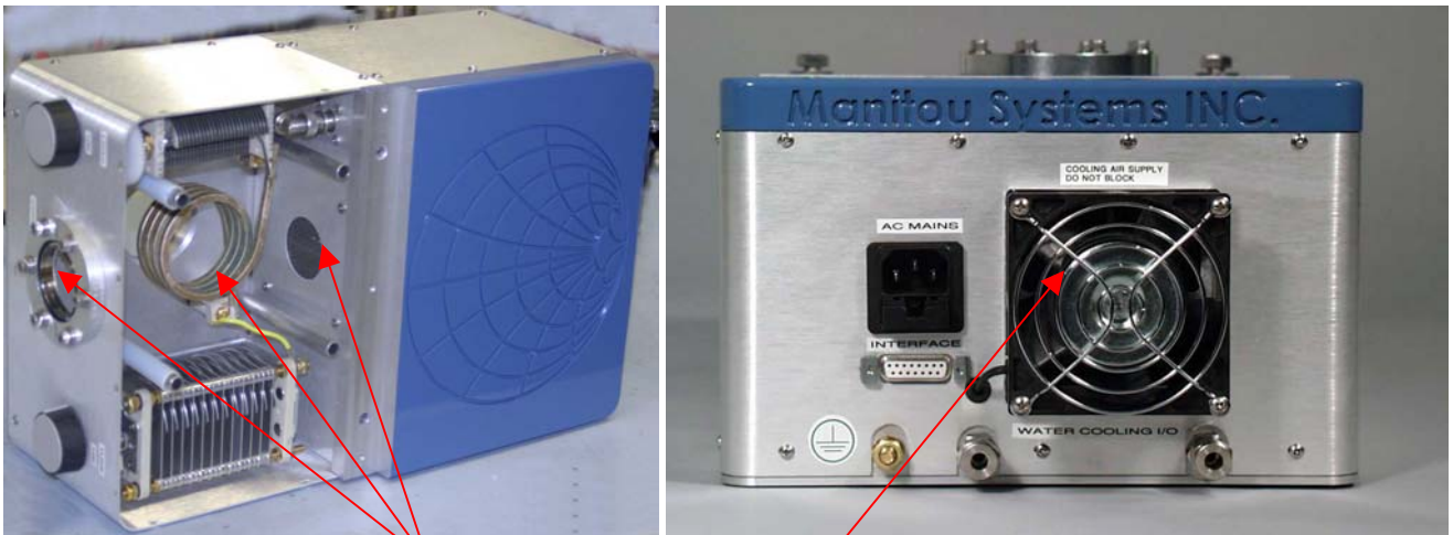
Clean dust and debris from these areas.
