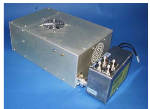
The image shown above represents a 2-way switch box installed on an automatic impedance matching network.
