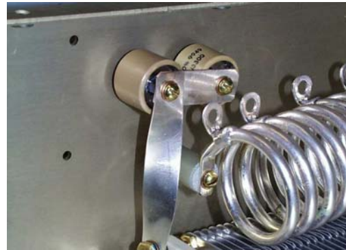
Fig. 3- Dual cap mounting location detail. (Note difference in angle of coil taps compared to fig. 2)
